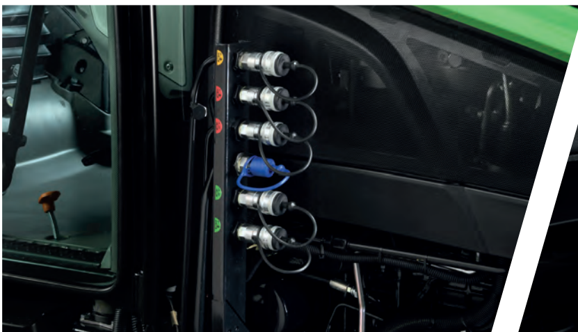
> Up to 5 mid-mounted hydraulic ways.
