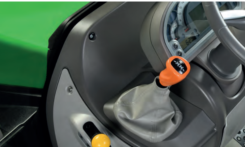
> Mechanical shuttle with ergonomic lever on steering column.
