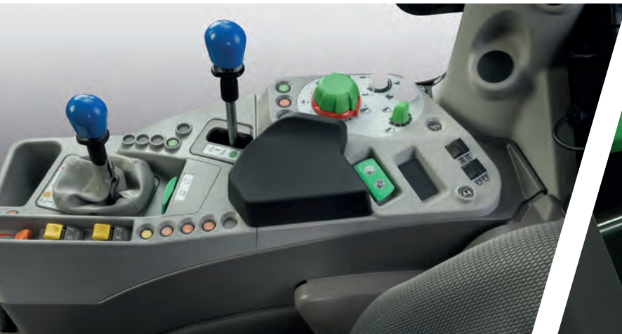
> Rear spool valves controlled by single levers or mechanical cross lever.
