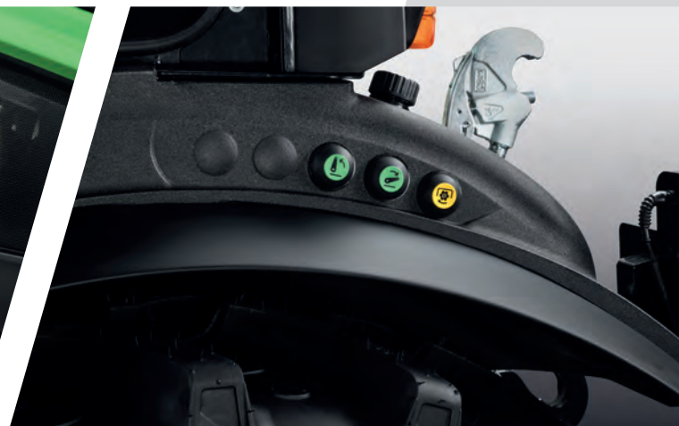
> External buttons for rear lift and PTO to make coupling manoeuvres easy.
