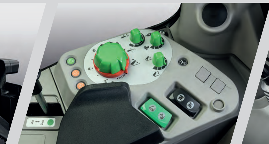
> Precise draft and position control thanks to electronic rear lift.
