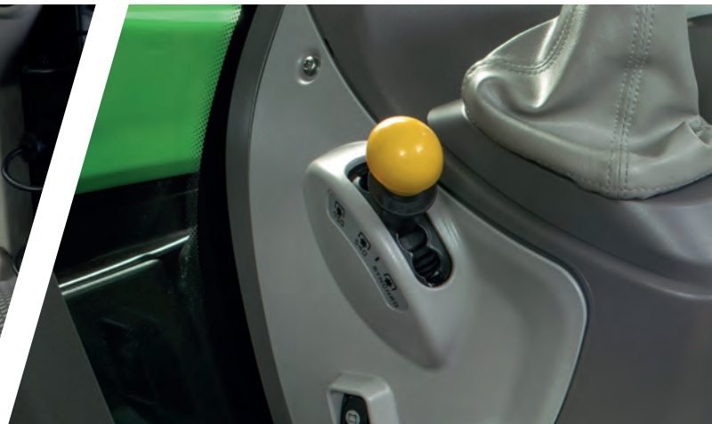
> In-cab PTO speed selector.
